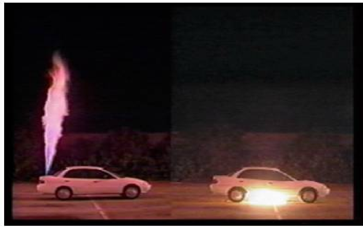
Photo 2 - Time 0 min, 3 seconds - Ignition of both fuels occur. Hydrogen flow rate 2100 SCFM. Gasoline flow rate 680 cc/min.
